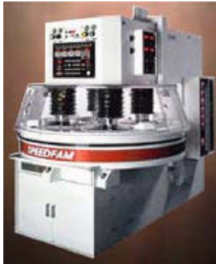
Fig. 2.5 Photograph of Speefam (Novellus) Multi Wafer per Platen Polisher [78]
